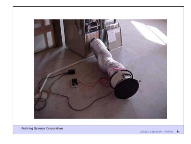
Duct Leakage Should Be Less Than 5% of Rated Flow As
