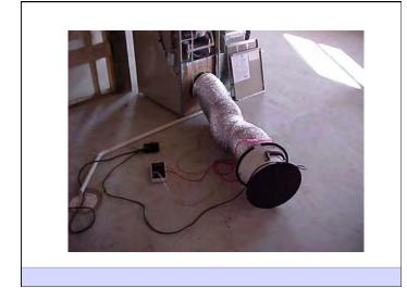
Duct Leakage Should Be Less Than 5% of Rated Flow As Tested by Pressurization To 25 Pascals
