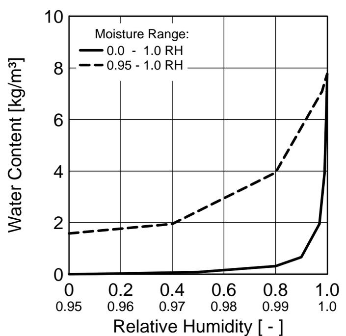
Material : Spun Bonded Polyolefine Membrane (SBP)
