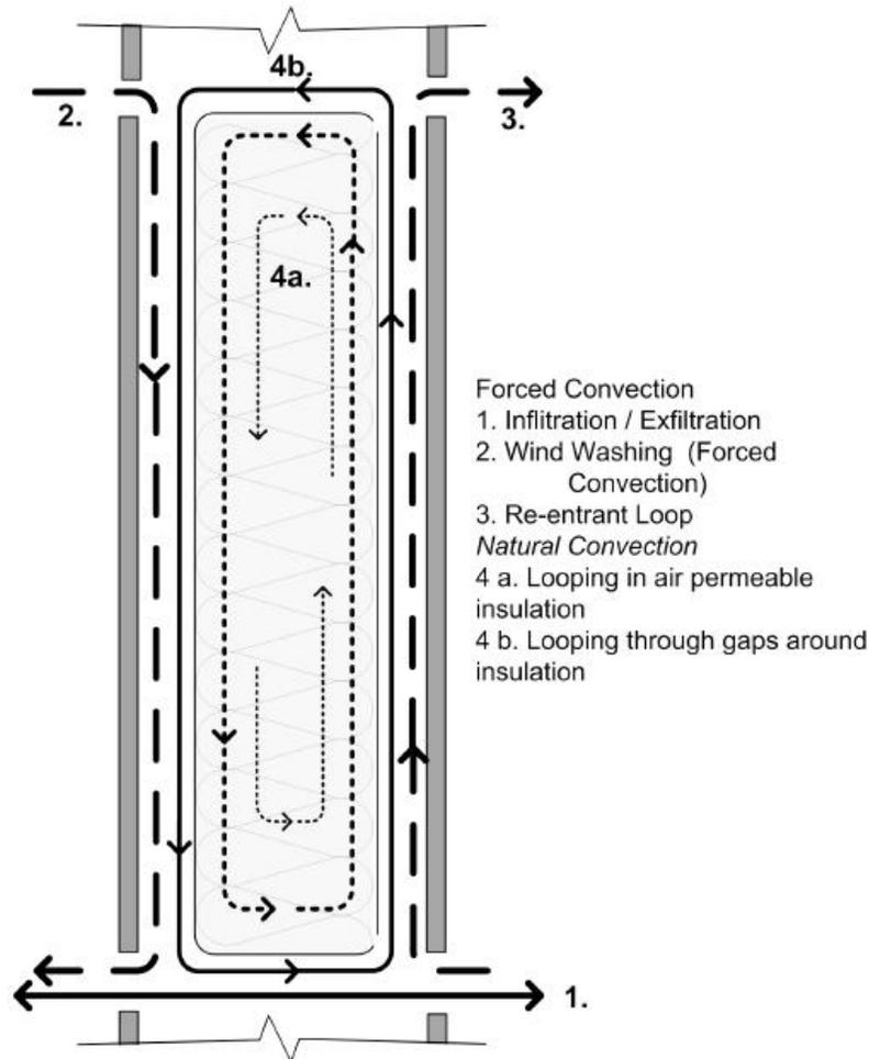
**Figure 5 : Common Convective Heat Flow Paths in Enclosures**
