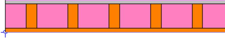
**Figure 7 : Actual average framing factor of 25% in standard construction**
