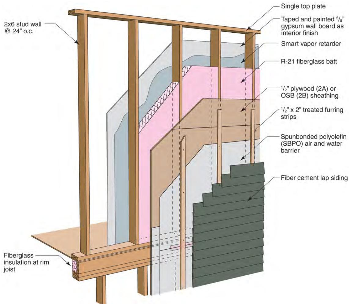
Figure 22 : 2x6 advanced framing construction
