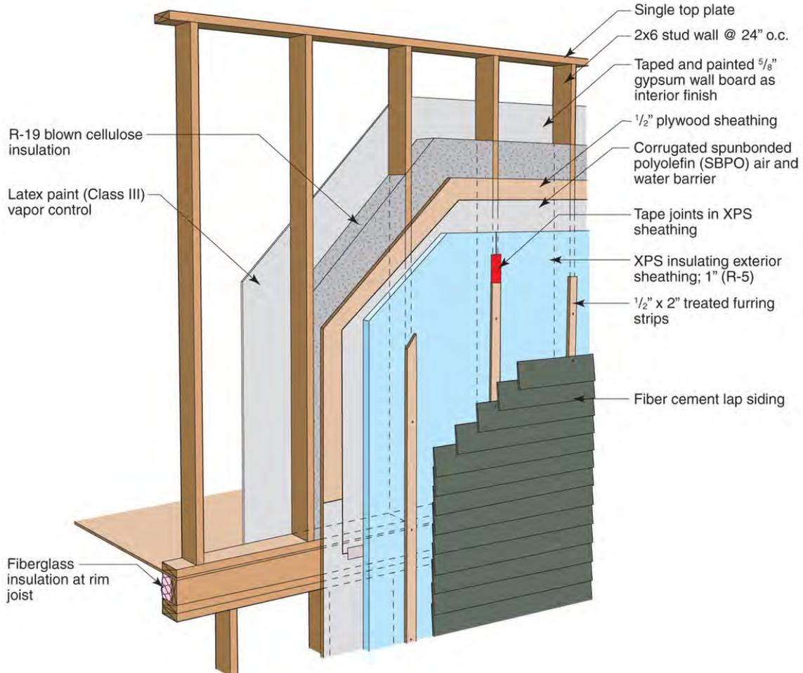
**Figure 26 : Advanced framing with cellulose cavity insulation and 1" of XPS exterior insulation**
