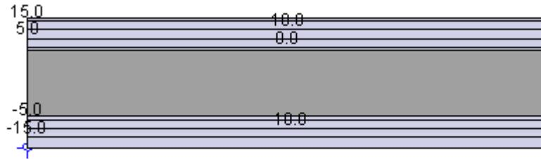
**Figure 48 : Eight inch foam ICF with four inches of EPS**
