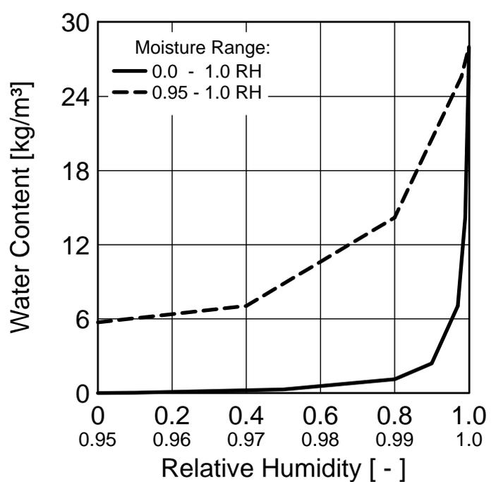
Material : Expanded Polystyrene Insulation (EPS)
