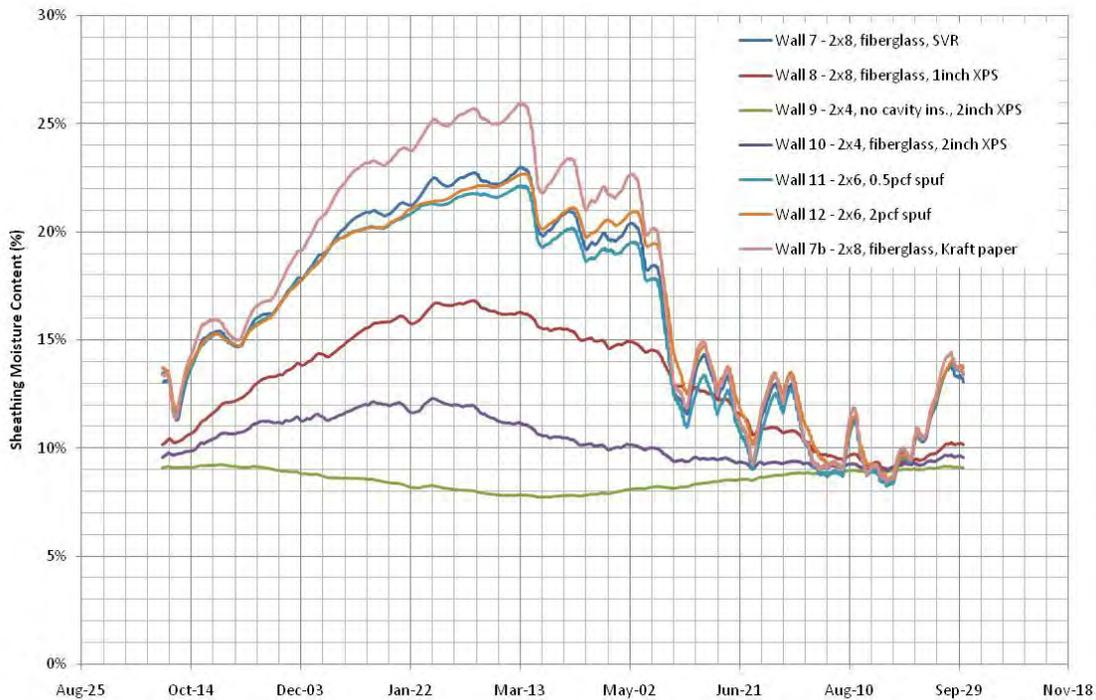
Figure 12 : Winter time sheathing moisture content for Walls 7 to 12
