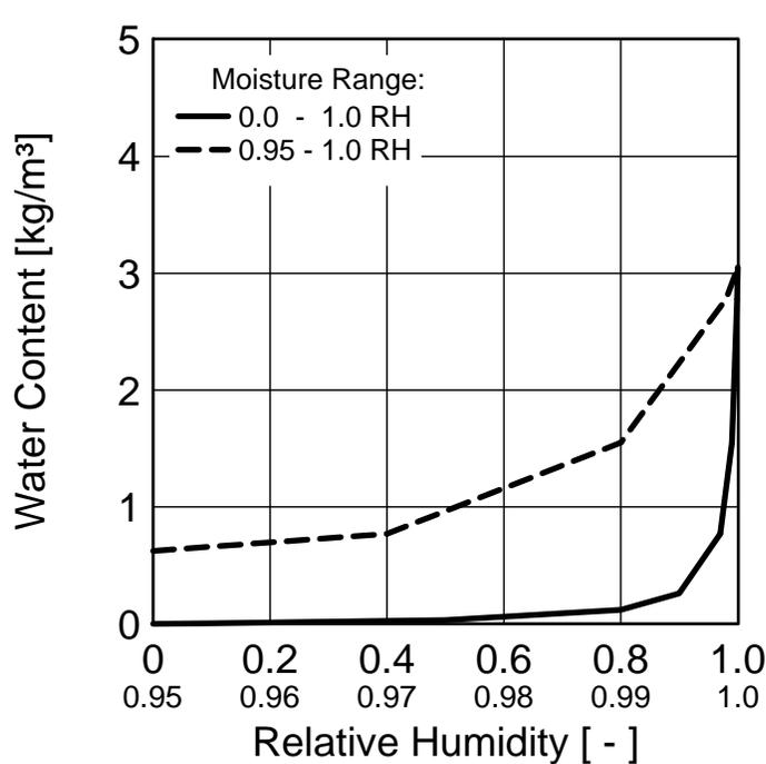
Material : Extruded Polystyrene Insulation (XPS)
