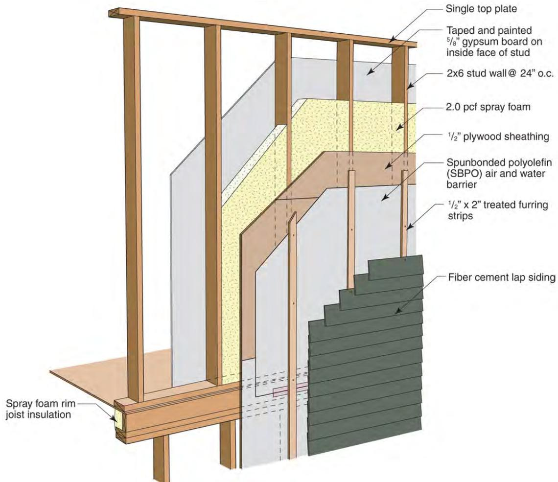
Figure 38 : 2x6 advanced framing with 2.0pcf Spray Foam
