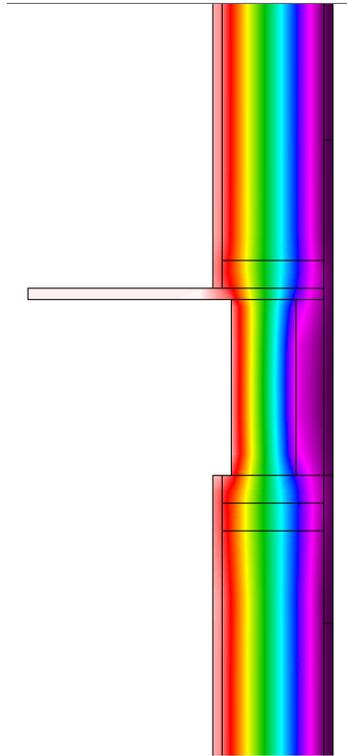
**Figure 41 : Therm modeling of Wall 13 – Advanced framing with hybrid cavity insulation (ie. Flash and Batt)**
