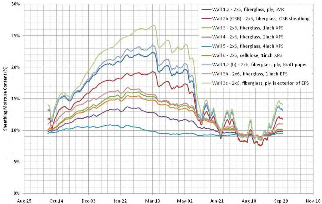
**Figure 9 : Winter time sheathing moisture content for Walls 1 to 6**
