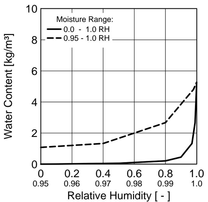
Material : Sprayed Polyurethane Foam; closed cell
