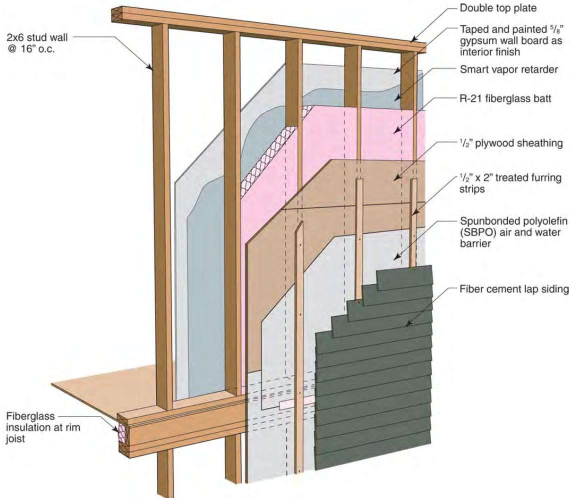
**Figure 20 : Standard 2x6 construction practice**
