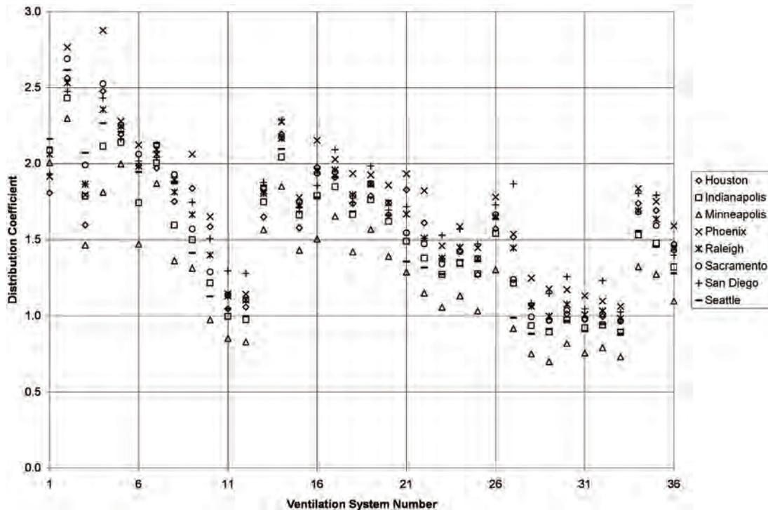
**Figure 10** System coefficients for exposure scenario A, 3.5 ACH50 houses.
