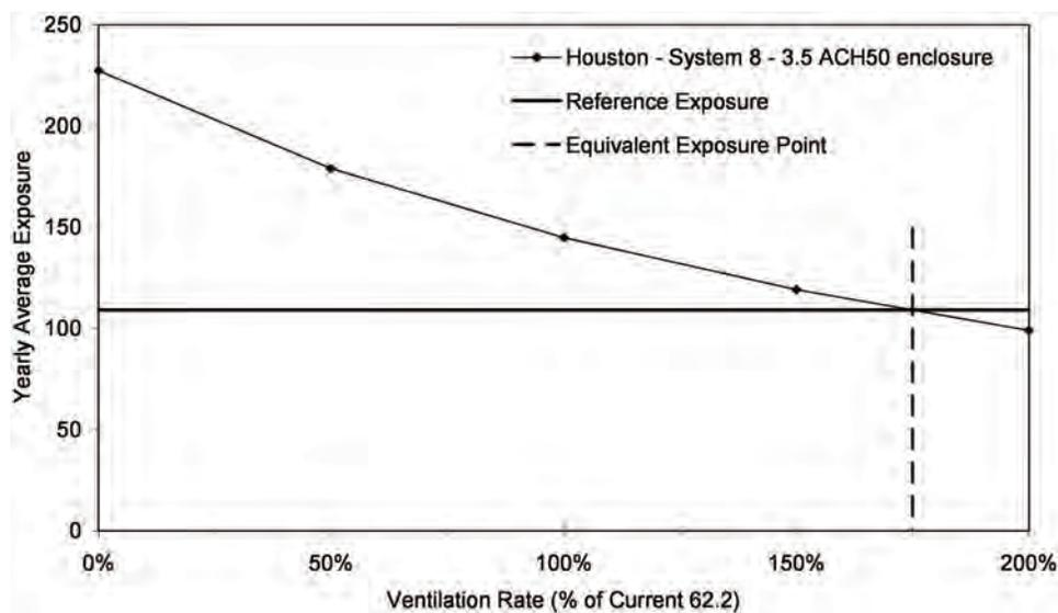
**Figure 9** Illustration of linear interpolation used to determine airflow required to achieve equivalent exposure to reference system, for ventilation system 8, Houston, 3.5 ACH50, and exposure scenario A.
