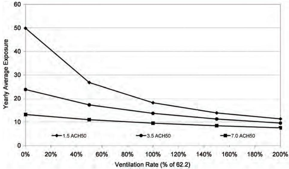
Figure 6 Effect of enclosure leakage rate.
