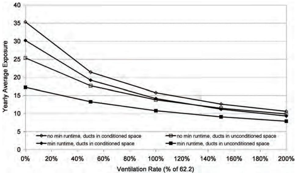
Figure 5 Effect of duct location and minimum runtime.
