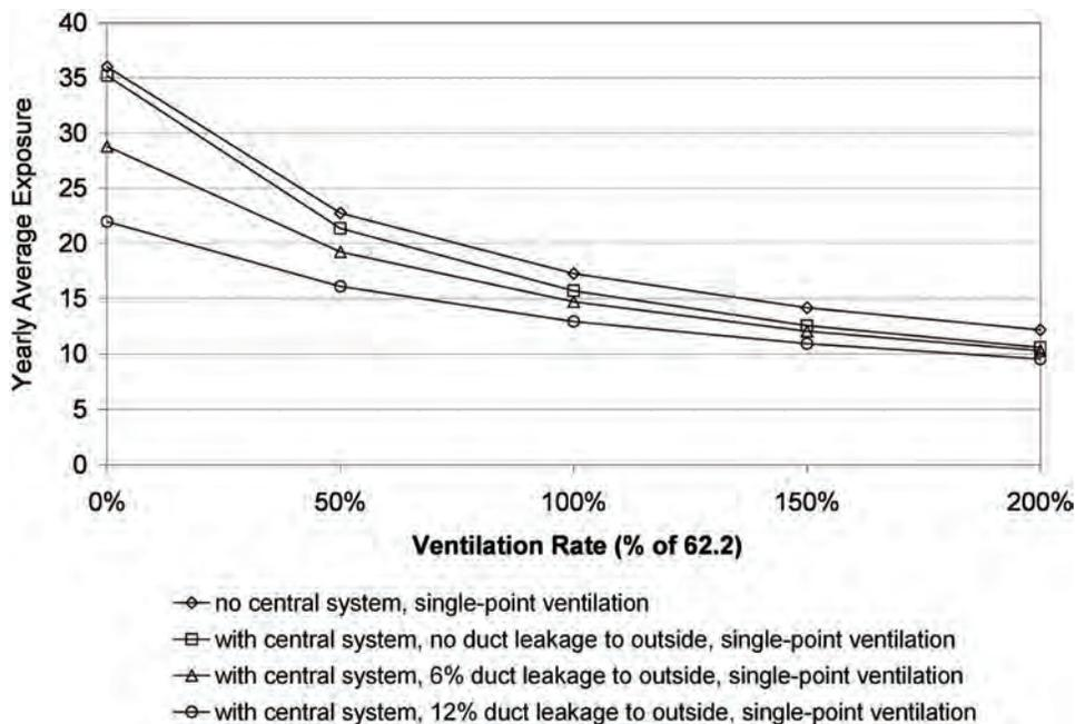
**Figure 3** Effect of central forced-air space conditioning system presence and location.
