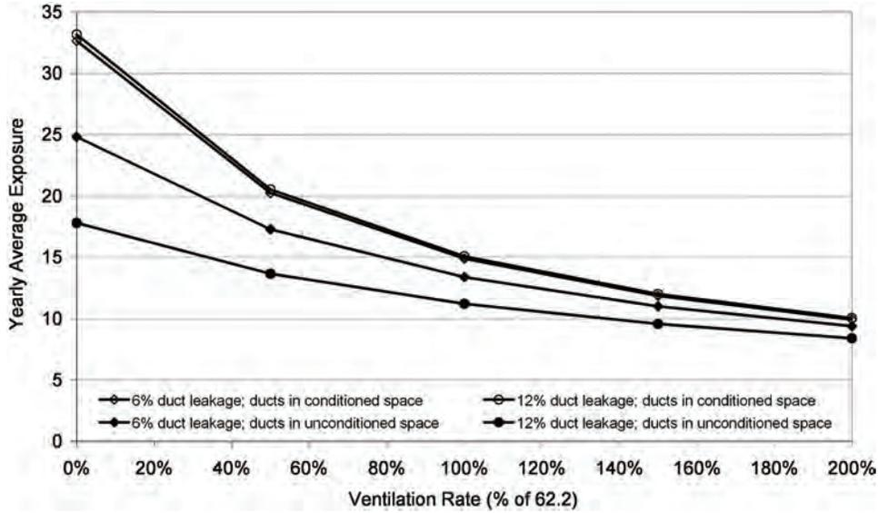
Figure 4 Effect of duct location and leakage rate.
