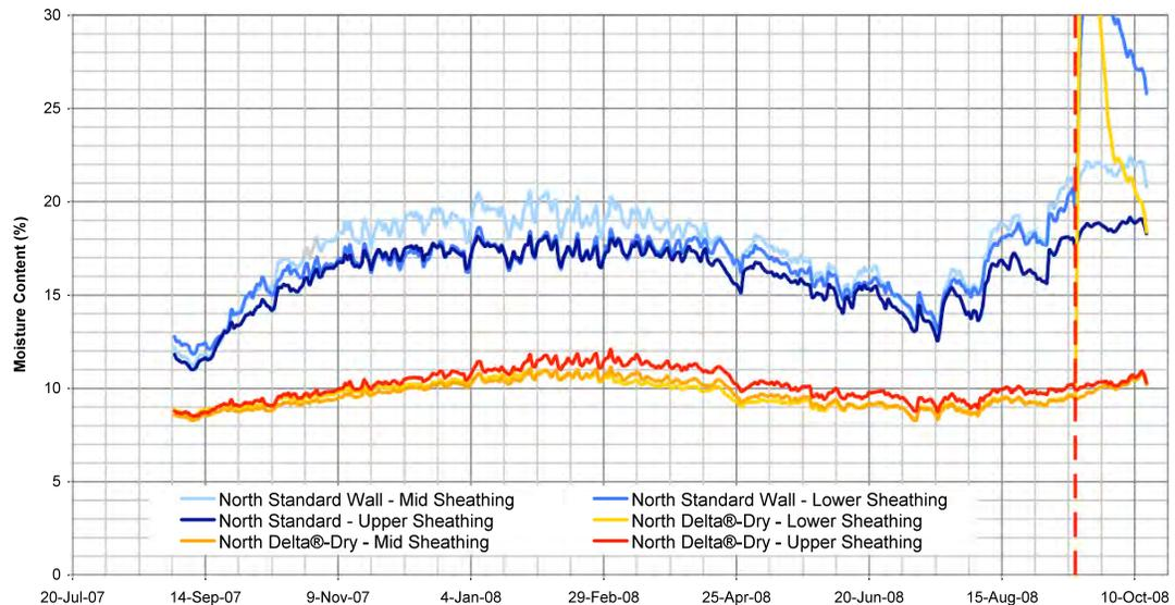
**Figure 5: Sheathing moisture content comparison on the north orientation**
