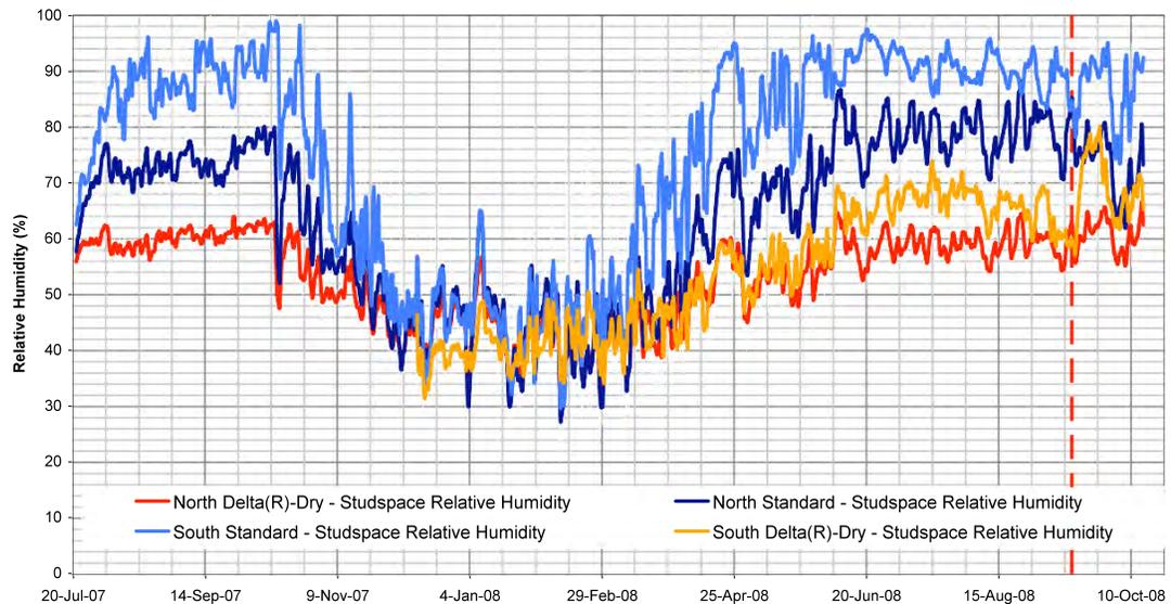
Figure 9: Relative humidity comparison of the stud cavities
