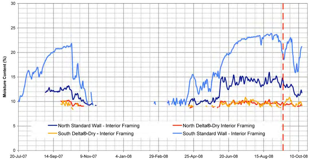
Figure 8 : Framing moisture content comparison of all test walls
