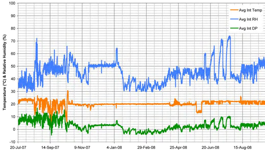
Figure 3: Interior Temperature and RH During Testing
