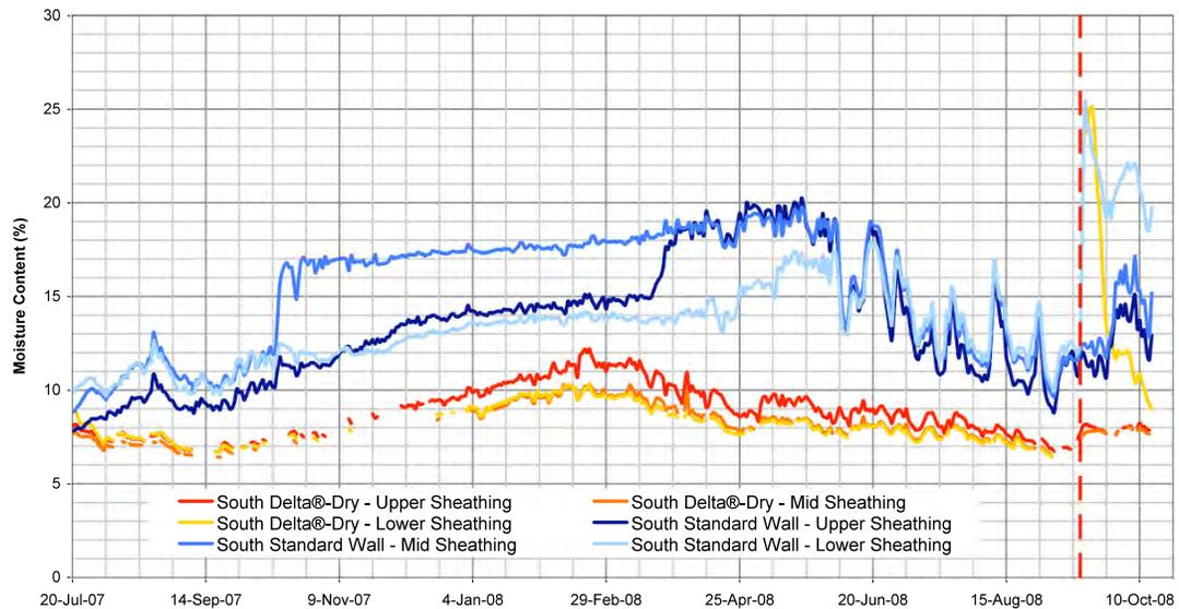
**Figure 6: Sheathing moisture content comparison of the south orientation**
