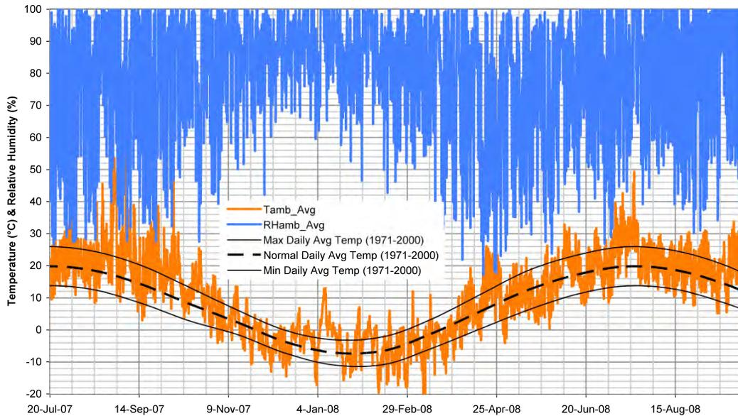
**Figure 2: Exterior Temperature and RH During Testing**
