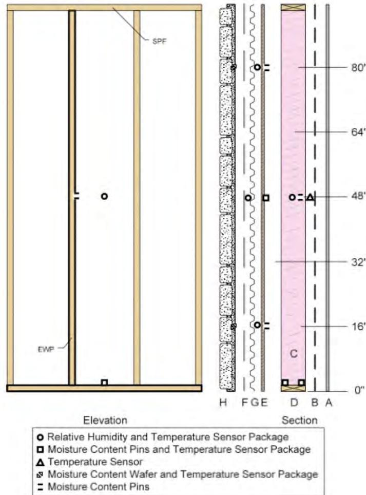
**Figure 1 : Typical Wall Construction and Sensor Layout For Full Scale Wall Testing**
