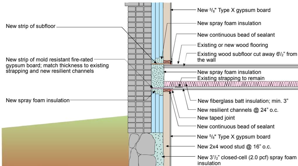
**Figure 9: Above-grade wall to below-grade wall transition**
