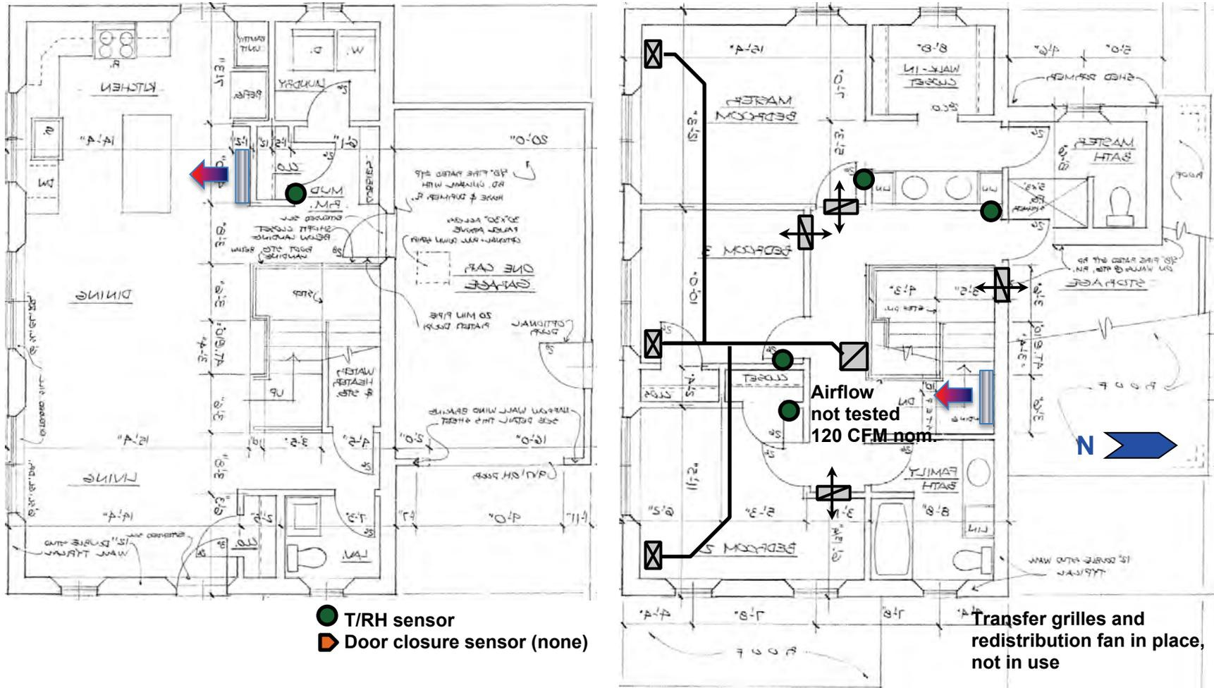
Figure 118. Easthampton Lot 13 floor plans, MSHP locations, monitoring locations
