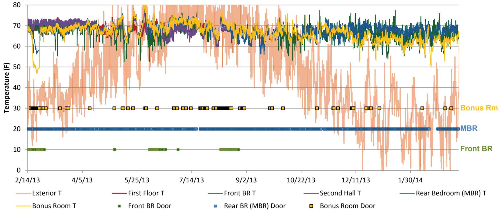
**Figure 129. Easthampton Lot 30 interior and exterior temperatures, with door closure status (over 50% closed hours)**
