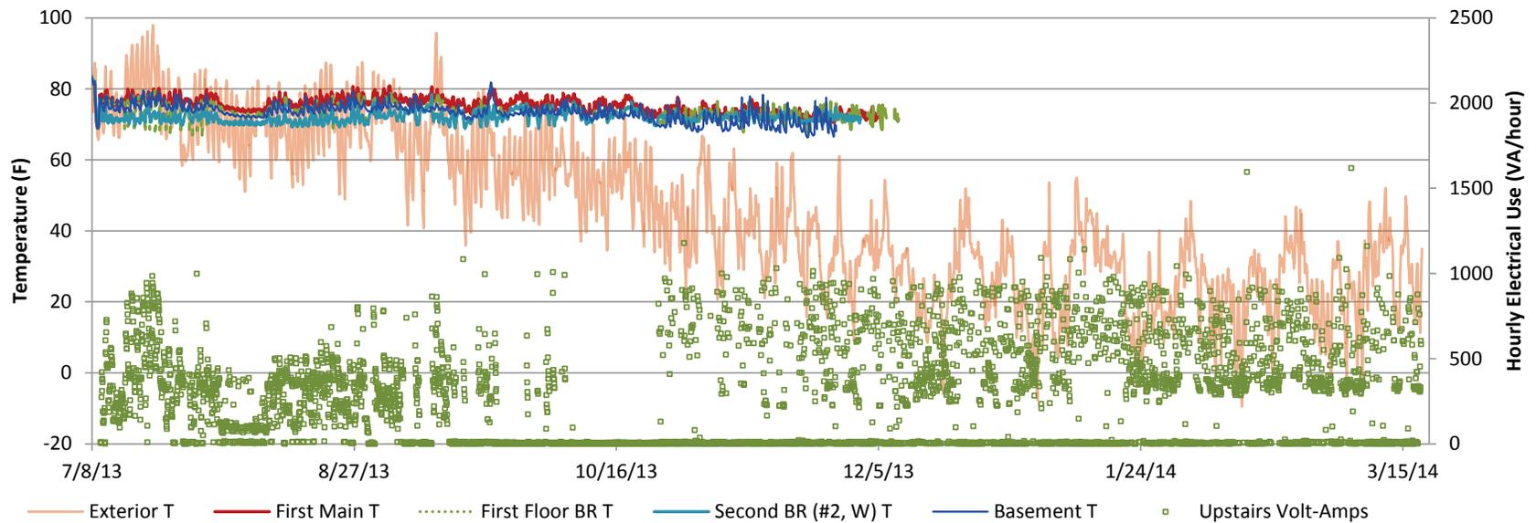
**Figure 113. Devens Lot 7 interior and exterior temperatures, with MSHP hourly electricity use (upstairs unit only)**
