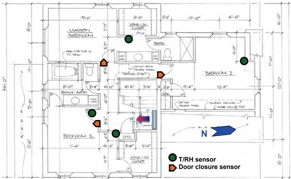
Figure 86. Second-floor plan, showing monitoring and MSHP locations
