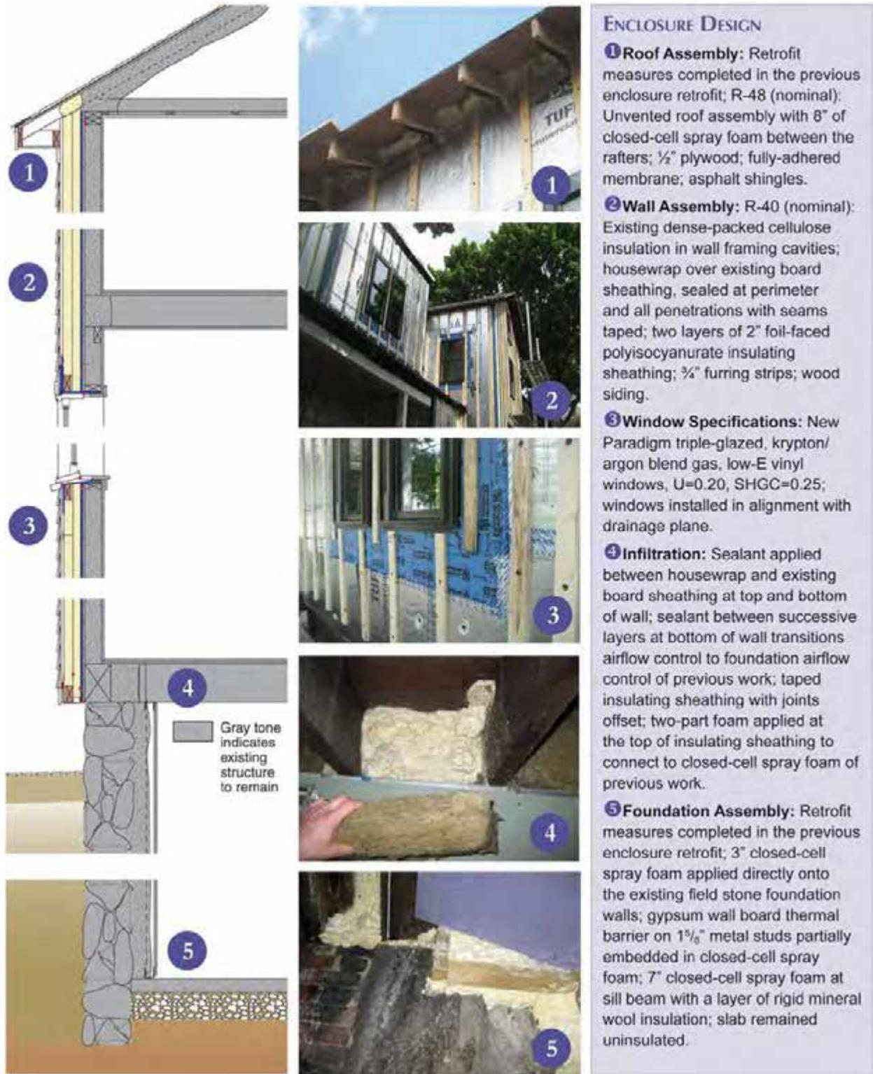
Figure A.11.2. Brookline DER Enclosure Profile
