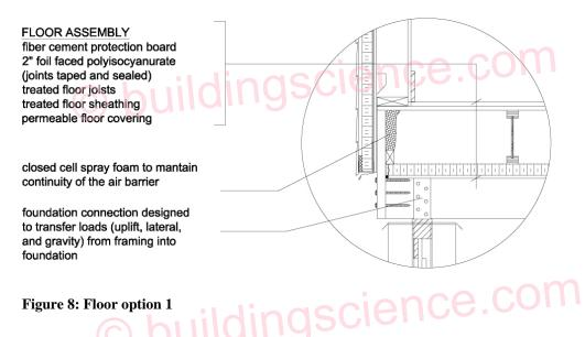
Similar to the roof assembly, the foil-faced polyisocyanurate can be replaced with closed cell spray foam provided that the floor finish installed over the subfloor is vapor semi-permeable. Open cell spray foam is not recommended for this application due to the high permeability of the material. With no exterior vapor control layer to prevent diffusion into the open cell spray foam, there is a concern of moisture accumulation under the floor material.
