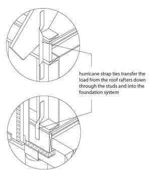
Figure 3: Hurricane ties used to create a load path through the structure
