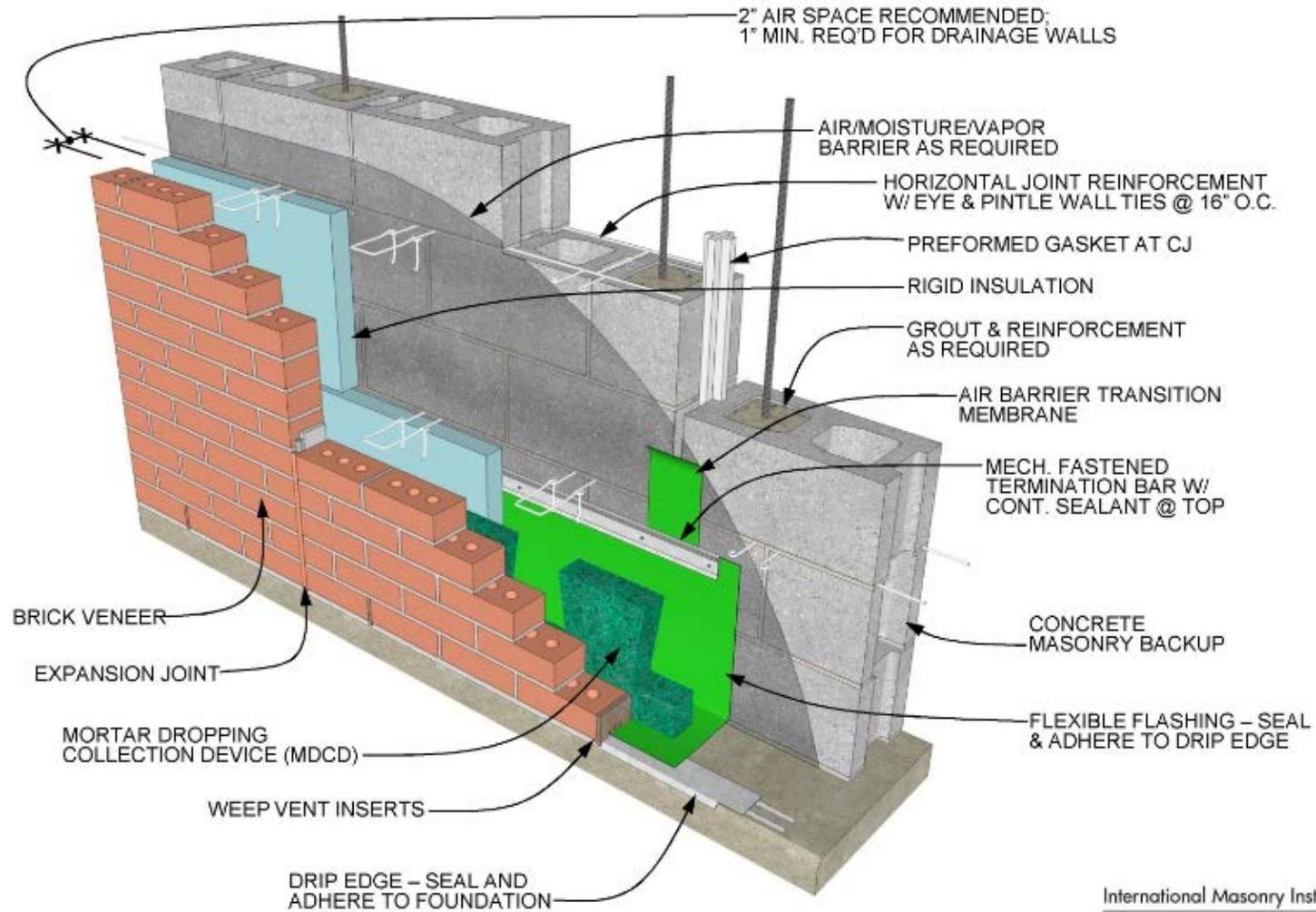
**BASE OF WALL DETAIL** FLASHING, DRIP EDGE, TERM. BAR, MOVEMENT JOINTS
