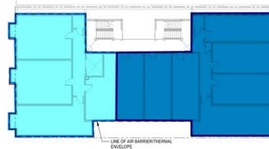
3 ENERGY CODE AIR BARRIER/THERMAL ENVELOPE PLAN - LEVELS 3-4 SCALE: 1/16" = 1'-0"
