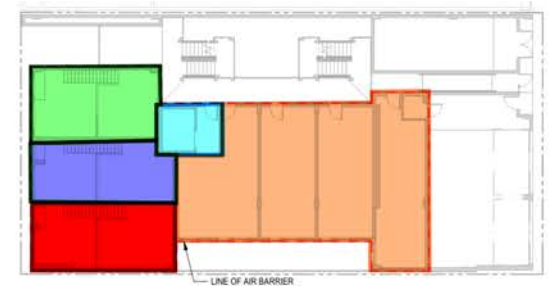
2 ENERGY CODE AIR BARRIER/THERMAL ENVELOPE PLAN - LEVEL 2 SCALE: 1/16" = 1'-0"
