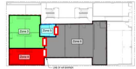
2 ENERGY CODE AIR BARRIER/THERMAL ENVELOPE PLAN - LEVEL 2 SCALE: 1/16" = 1'-0"
