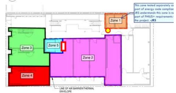
1 ENERGY CODE AIR BARRIER/THERMAL ENVELOPE PLAN - LEVEL 1 SCALE: 1/16" = 1'-0"
