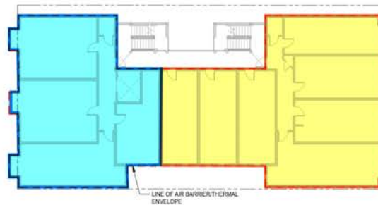
4 ENERGY CODE AIR BARRIER/THERMAL ENVELOPE PLAN LEVELS 5-7 SCALE: 1/16" = 1'-0"
