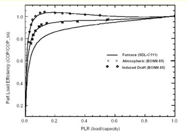
Figure 6: Recommended Curves for Furnaces and Boilers
