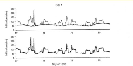
Figure 2. Measured and modeled infiltration at Site 1. The bold line in the upper graph is the adjusted natural infiltration prediction; in the lower graph it is the adjusted infiltration combined with the fan model.
