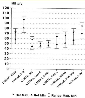
Figure 4-1. HERS BESTEST Tier 1 example range setting—annual heating load (L100AC through L170AC) for Colorado Springs, CO
