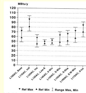
Figure 4-1. HERS BESTEST Tier 1 example range setting—annual heating load (L100AC through L170AC) for Colorado Springs, CO
