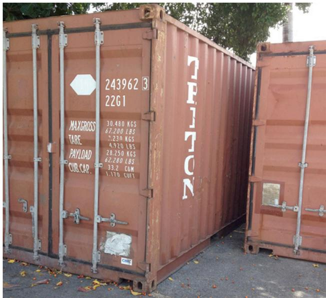
**Photograph 2: Tantlinger’s Box** – Note the corner castings built into the eight corners of the shipping container. A rotating connector “twistlock” locks into the corner castings. The “double cone” twistlock became a staple in the shipping and transport industry and “stack and lock” containers dominate to this day. The ability to stack the boxes and
