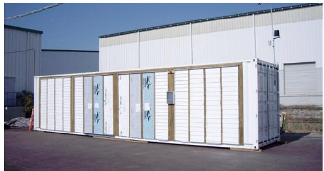
**Photograph 6: Mobile Hygrothermal Test Bed** – designed, constructed and instrumented by Building Science Consulting, Inc. out of Waterloo, Ontario.
