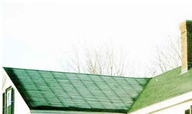
**Photograph 4. Thermal Bridging—**Guess whose house that was? Yup. It was mine. I am not as smart as I think I am most of the time. At the time this photograph was taken the underside of the roof was insulated with closed-cell spray polyurethane foam (SPF).
