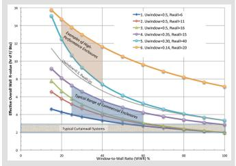
Typical curtainwall systems have an R-value of only 2 or 3, with "high performance" systems (not shown) using highly insulated (say R-12) spandrel panels and best-in-class double glazing (with low-e and Argon) may achieve R-4. Only a few systems, such as the Kawneer 7550 series or Visionwall, can achieve R-values of 6 or more.
