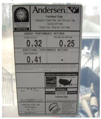
The U-value is the reciprocal of the R-value. A U-value of 0.33 is an R-value of 3 for example, (except that in the case of glazing systems the U-value includes the effect of surface films, unlike walls). As the climate becomes cold or very hot, a low U-value becomes important for energy savings and for comfort. Buildings with low U-value windows and/or curtainwalls can dispense with special, and costly, perimeter heating even in very cold climates.
