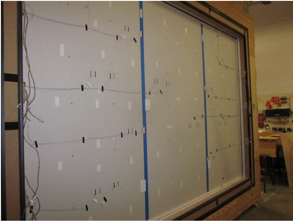
Figure 24 – Meter Box Side, Grid of Double-Sided Tape
