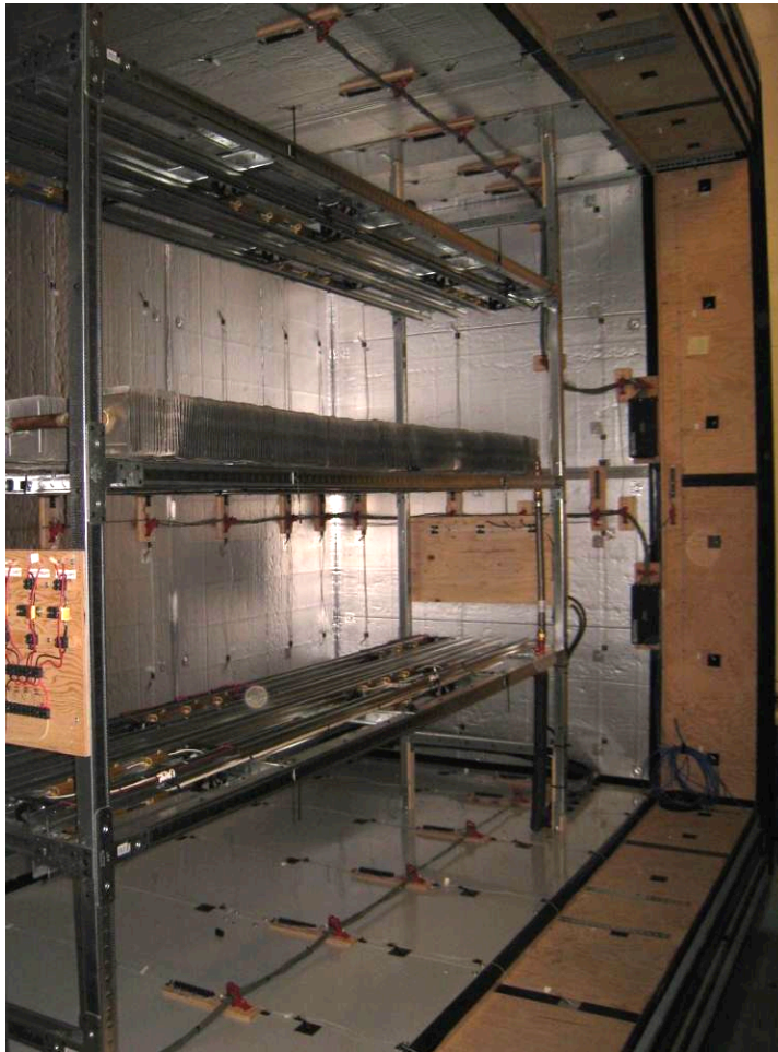
Figure 2 – Upper and Lower Heating Arrays with Cooling Coil in Meter Box
