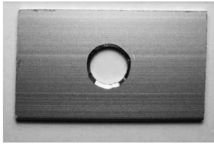
Figure 12 – 1/16" Aluminum Stock Spacer
