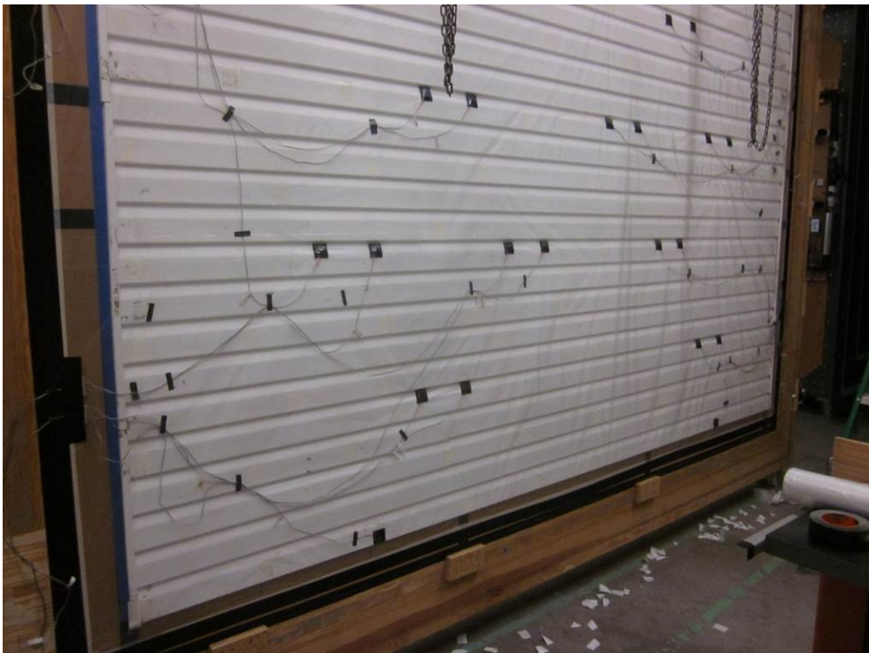
Figure 27 – Climate Box, Polyethylene Installed
