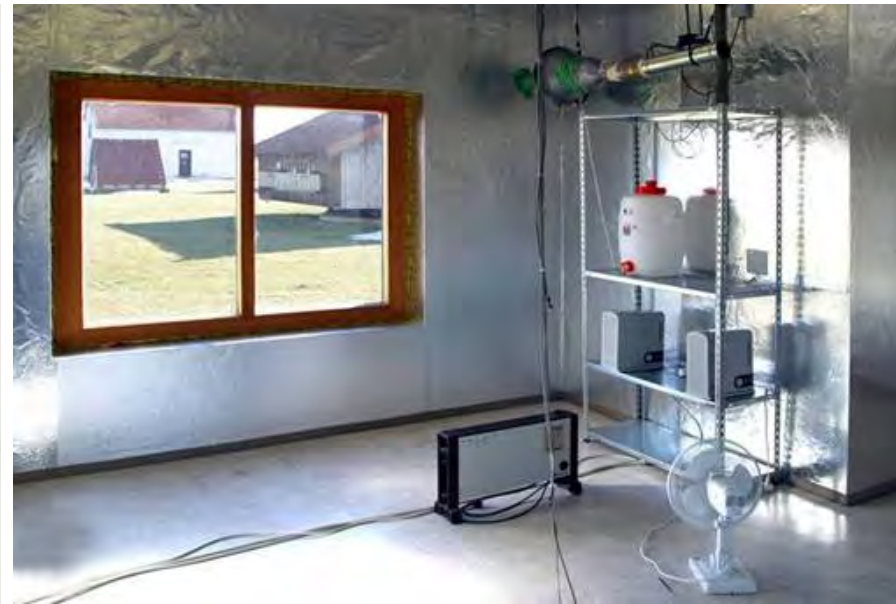
Interior lining test room with aluminum wall paper
