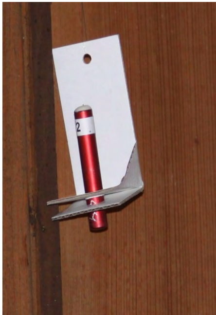
© Fraunhofer IBP Source: Fluid Tracergas A / B; Constant Tracergasemission by PENTIAQ, Sweden
