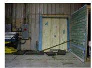
Stud penetrated cladding but not through Wall 1
