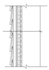
Wall 2 (Wall 1 + high density closed cell spray foam)
