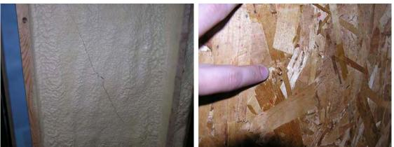
Figure 11: Cracking of both Closed Cell Foam and OSB Sheathing at 40 fps
