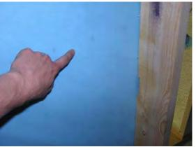
Figure 17: No penetration of Wall 1 at 30 fps
