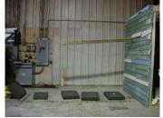
Stud penetrated cladding but not through Wall 2
