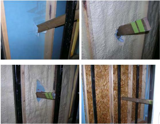
Figure 8: Stud penetration through all wall assemblies at 50 fps
