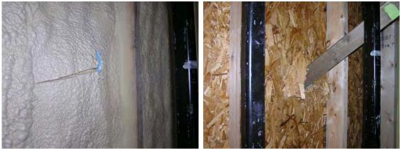
Figure 14: No penetration of Wall 2 and penetration of Wall 4 at 43 fps
