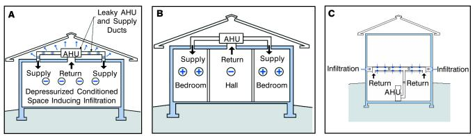
Figure 1: HVAC system-induced air changes occur via: (A) leaky ductwork and AHU located outside of the building; (B) unbalanced airflows due to door closure and inadequate return flow; (C) air pressure effects within building activities.
