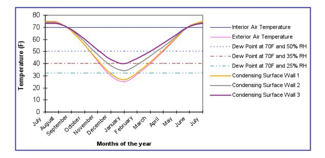
In reality, the exterior temperature can vary quiet significantly from the monthly averages potentially leading to events of condensation occurrence.
