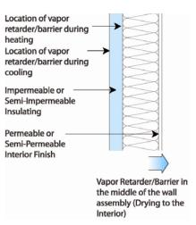
The thermal gradient can be predicted by examining the individual proportion of thermal resistance provided by each component. Each different component will provide a percentage of the total thermal resistance of the assembly. Therefore, the change in temperature of any component is based on the percentage of thermal resistance provided by that component multiplied by the overall temperature difference across the assembly.
