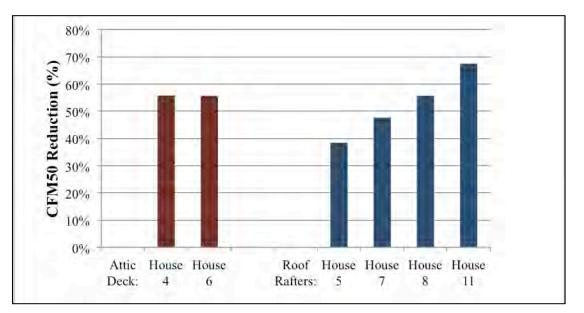
Figure 27. Air leakage reduction for attic deck and roof rafter strategies
