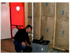
As would be expected with the The total air distribution system leakage distribution system entirely within a very was higher than expected given the airtight enclosure, system testing found obvious attention to duct sealing by the no measureable leakage to the outside.
