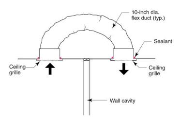
**Figure 2a: Jump Ducts** – This addresses the problem in Figure 1b. What is nice about this approach is that it is quiet – no sound transfer. Also known as a "slinky".
