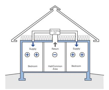
**Figure 1b: Even More Negative** – When you then install systems with central returns that are also unbalanced in that return paths are not provided from bedrooms to the central returns the pressure effects are magnified. Undercutting doors does not work unless you have a "knee high" undercut.
