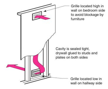
Figure 2b: Transfer Grilles – This also addresses the problem in Figure 1b. Less expensive than a "jump duct" but not as quiet.
