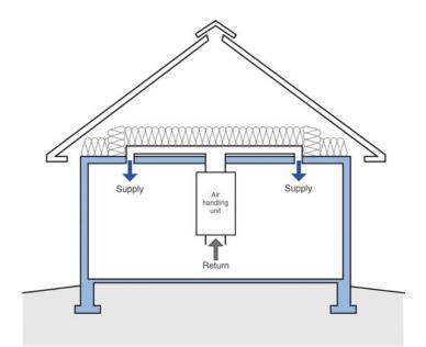
**Figure 3e: Buried Ducts** – Take the John Tooley option, make the ducts airtight, make the ceiling airtight and insulate the bejesus out of the ducts by covering them with lots of "fluffy stuff". You can cut that 10 percent hit to less than 5 percent.
