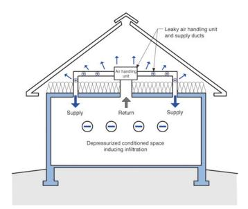
**Figure 1a: Really Negative** – Ductwork and air handlers typically leak and when the are installed outside of the conditioned space such as in a vented and unconditioned attic significant negative pressure occur inside of the conditioned space that lead to significant energy penalties in all climates and large latent loads in humid climates.
