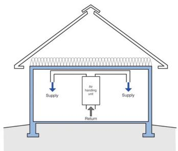
**Figure 3a: Base Case** – The best of the best. Ductwork and air handler inside the conditioned space with a vented attic on top with an airtight ceiling and code levels of attic insulation. It does not get better than this anywhere anytime.
