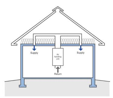
**Figure 3c: Less Ugly** – The moment you put the ductwork in the attic (while keeping the air handler inside) having this ductwork airtight (installed by John Tooley himself) with an airtight ceiling (installation watched over by me) all penetration and boots and stuff sealed you still have about a 10 percent energy hit on cooling and heating compared to the base case. This is much better than Figure 3b but it sure ain't Figure 3a.
