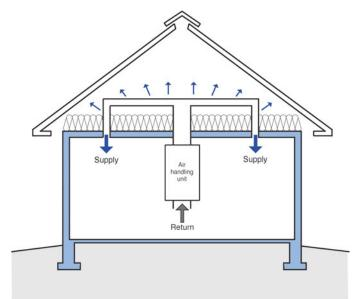
**Figure 3b: Ugly and Unfortunately Typical** – This is a 30 percent or more energy hit on cooling and heating compared to the base case.
