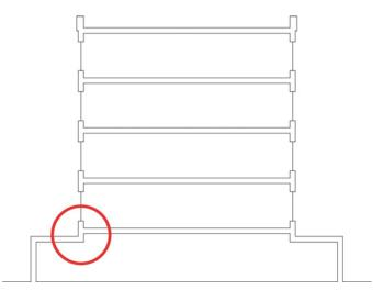
**Figure 5: Elevated Slab**—Common way of building apartments and condos with a parking garage underneath that is unconditioned. The red marks the spot. You can only insulate on the top or on the bottom. None are fun if you are serious about the thermal bridge caused by the slab sticking out horizontally "all over."
