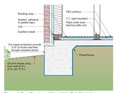
Figure 4: Post-Tensioned Monolithic Slab Brick Veneer—
