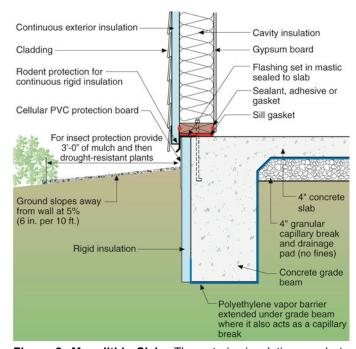
**Figure 2: Monolithic Slab**—The exterior insulation needs to be protected during construction and it has to be protected during its useful service life. And don't forget about the capillary break and insects. This works only for moderately bad dirt.
