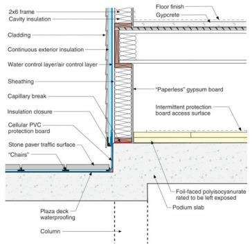
Figure 8: Conditioned Crawlspace—Easiest to construct but complicates life with respect to "access" due to the finished floor being located above the podium slab. The crawlspace has to be conditioned and compartmentalized. The crawlspace is a good place for ducts and plumbing.
