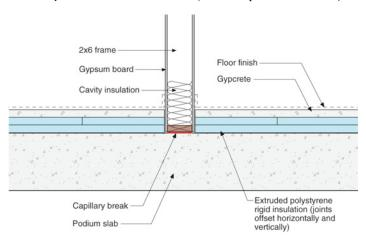
**Figure 7: Top Side Interior**— Note the liquid gypsum floor leveling system that provides fabulous fire protection and acoustical properties (aka "Gypcrete"). It does something else for us that reduces risk – it makes the floor pretty much "spill proof". Nothing gets through it.
