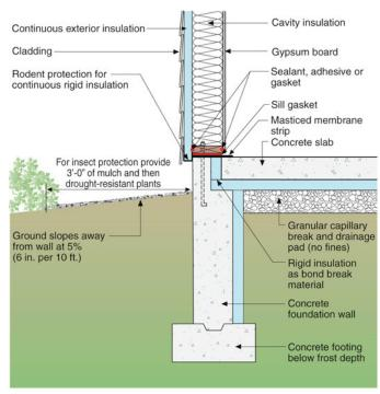
Figure 1: Insulated Stem Wall—With good soil conditions construct the foundation assembly out of three pieces – a footing, a stem wall and the "flat plate" slab part. Insulate it under it and on the inside of the perimeter making sure you uncouple the plate from the stem wall at its edge. This edge thing is a big deal – the thermal bridging that occurs if you don't do it costs you more than half the thermal resistance of the whole deal.
