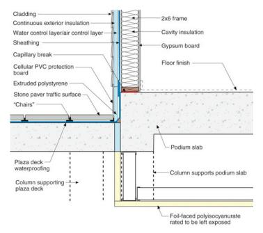
**Figure 9: Bottom Side Approach**—Columns are still thermal bridges that can be a real problem in very cold climates like climate zone 8 and climate zone 9 – in which case small heaters are added to this space or the columns wrapped with "heat tape."
