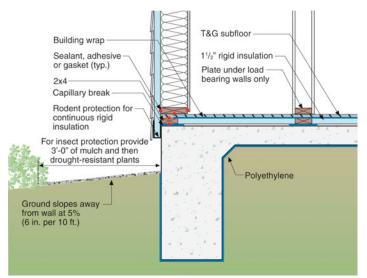
Figure 3: Post-Tensioned Monolithic Slab—Elegant and ugly. Elegant because it works. Ugly because you can't let it get too wet during construction which is a problem because we build outside. And when it gets wet during construction you need to let it dry before you cover it.
