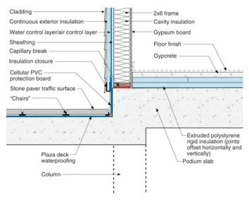
**Figure 6: Top Side Perimeter**—The "fill in" approach. It allows the slab to be open during much of the construction process and sequences the insulation and subfloor installation such that it occurs after "dry in".
