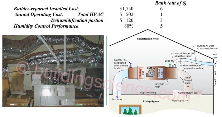
System description The enhanced dehumidification with cooling and central-fan-
