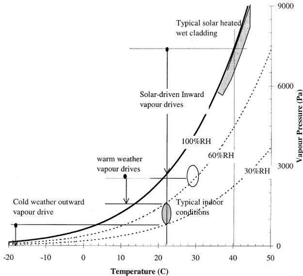
**Figure 2** Vapor pressures in and around enclosure walls.
