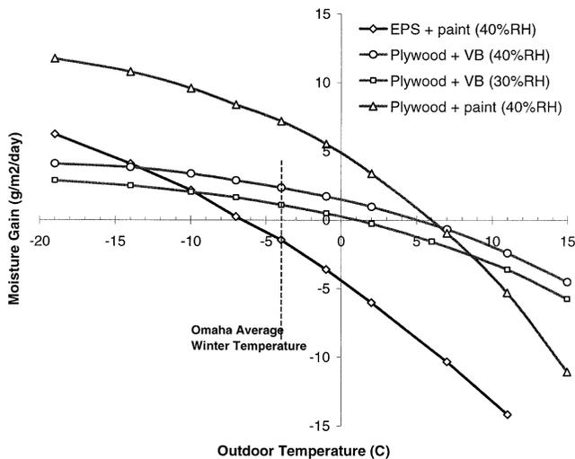
**Figure 1** Impact of exterior temperature on condensation rate.
