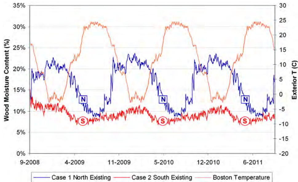
Figure 8 Existing wall with 0.5% of incident rain penetration, north and south exposures, with exterior temperature for reference (seasonal patterns).
