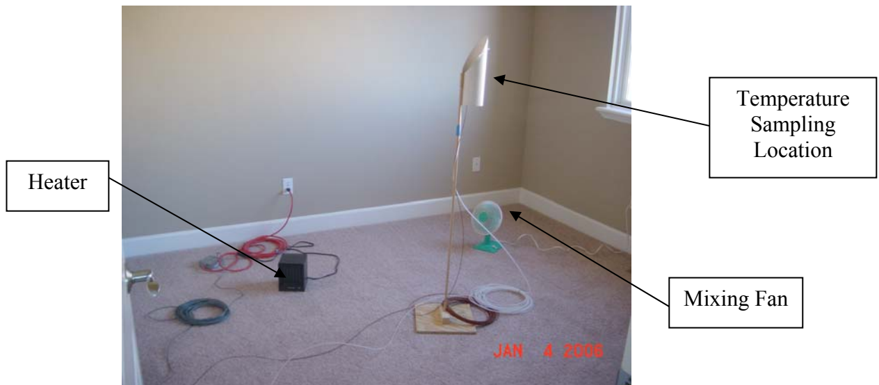
Figure 6. Tracer gas sampling point, temperature sensor, room air mixing and co-heating set-up.
