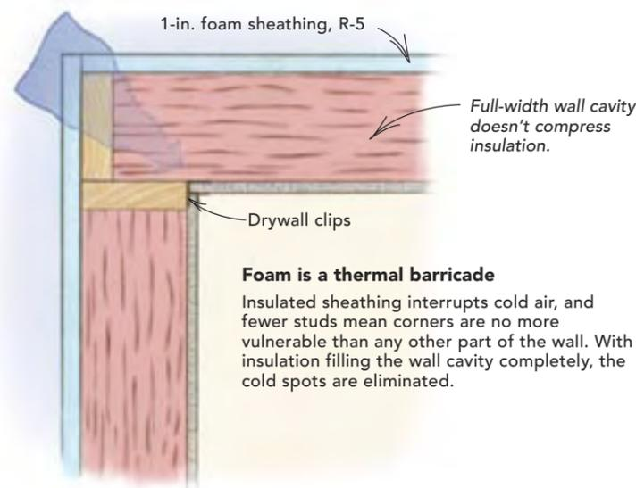
framing increases joist, stud, and rafter spacing to 24 in.; places doors and windows on stud layout; and demands that framing members be lined up (or stacked) for direct load transfer. Coupled with better insulation detailing, those same smart-framing strategies also can reduce the cost of heating and cooling houses.
