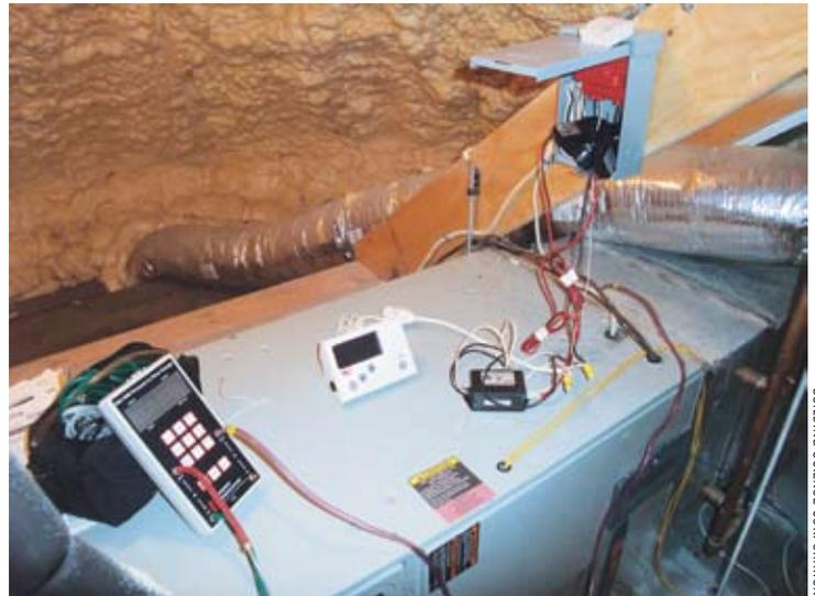
Measurement procedure, showing digital manometer (Energy Conservatory DG-700) and power meter (The Energy Detective). TrueFlow airflow measurement plate is inside filter slot.
