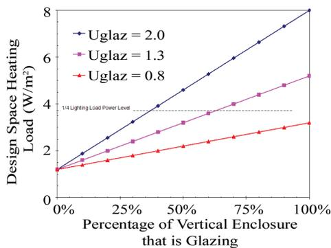
Figure 3 – A closer look at Space Heating Load Requirements as a Function of Glazing U-value and Area Heating and Cooling. Design Heating Load based on outdoor temperature of -4F (-20C) and an average of 32.8 ft (10 m) distance from enclosure to center of building.
