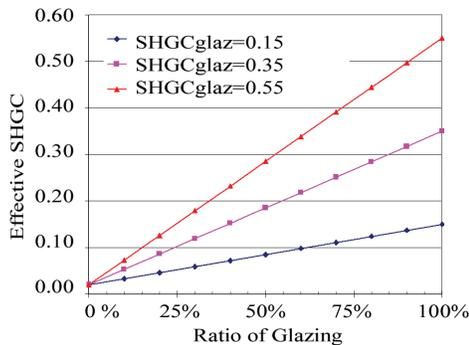
Figure 2 – Effective SHGC as a Function of Glazing Area and Glazing SHGC Natural Ventilation.
