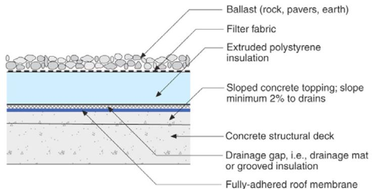
**Figure 3: PMR and IRMA**—Protected membrane roofs and inverted roof membrane assemblies date back in North America to before I was born—a time when the Toronto Maple Leafs were winning Stanley Cups. Note that drainage below the extruded polystyrene (XPS) layer is necessary to keep it from becoming saturated over time.
