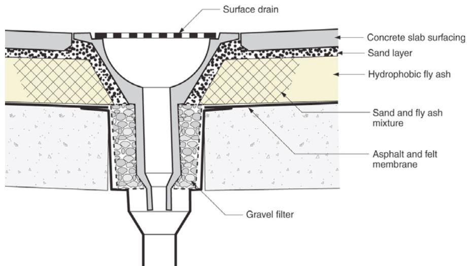
**Figure 2: More Soviet Era Stuff**—Great roof drain. Could have also been the design for a shower drain. For real, not kidding.
