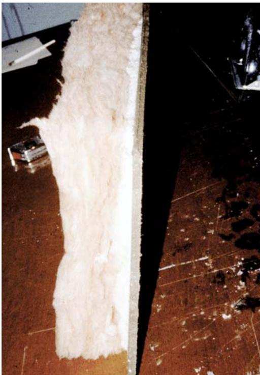
**Photograph 1: Surfaces are Where the Action Is**—The frost has accumulated at the backside of the sheathing, not in the middle of the cavity insulation.
