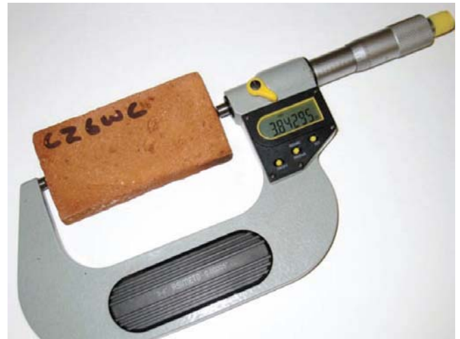
Photograph 1: Measuring Brick Expansion Under Freeze/Thaw Cycling —A micrometer is used to determine permanent irreversible expansion. The moisture content of the brick at which, under repeated freeze/thaw cycles, results in permanent irreversible expansion is called the "critical degree of saturation."
