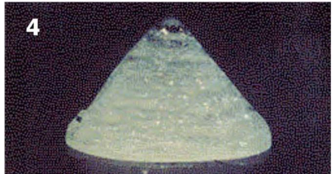
**Photograph 2: Frost Heaving in the Lab** (A sequence of Photographs courtesy of the American Physical Society from a paper by Ozawa, H. 1997. "Thermodynamics of frost heaving: A thermodynamic proposition for dynamic phenomena," *Physical Review E* 56(3):2811 – 2816).
