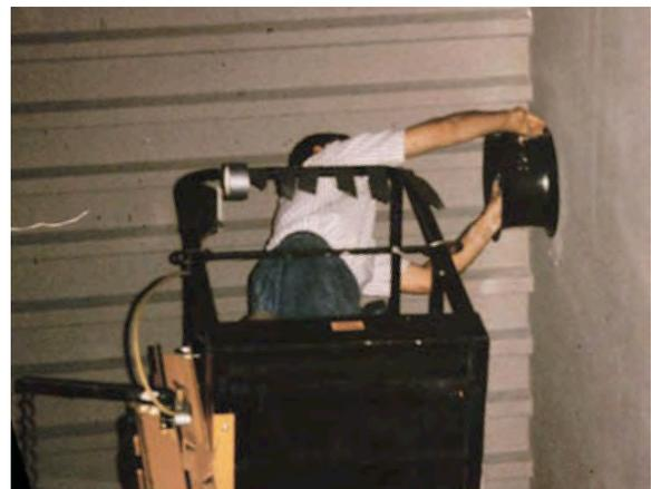
**Photograph 11:** Duct Blaster® pressurization of parapet assembly.
