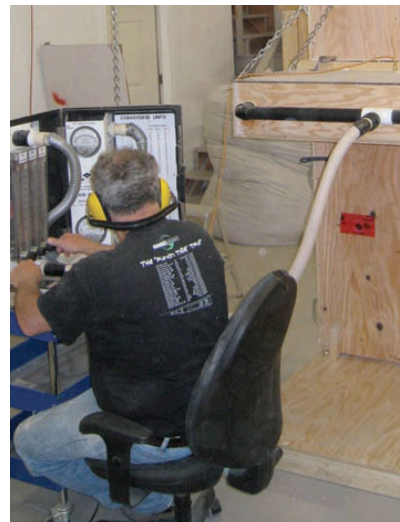
Photograph 3: Skunk Works Air Leakage Testing —Applying air pressure and measuring flow. There's nothing magical here. But, the results are impressive.
