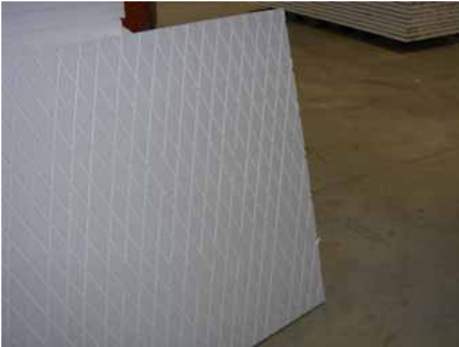
Photograph 10: Groovy —Cross-cut grooves in the back of foam sheathing to provide relief of hydrostatic pressure and lateral hygric redistribution.
