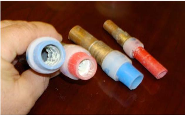
**Photograph 5: Meringue Dezincification**—Note the corrosion product, zinc oxide residue, blocking the fitting.
