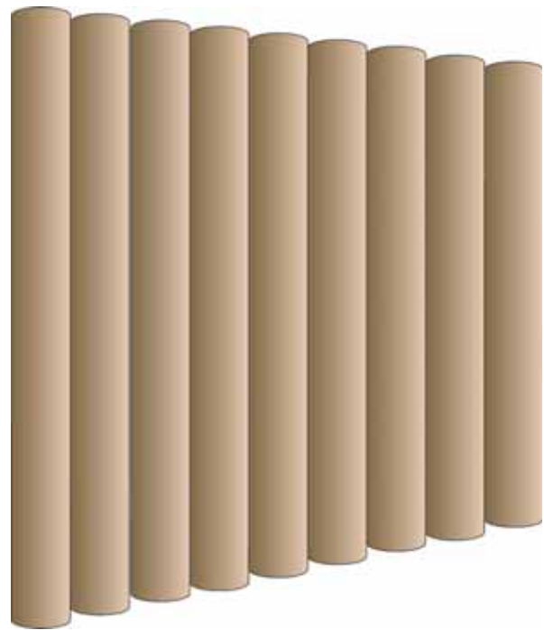
Palisade wall: Closely spaced posts embedded in the ground
