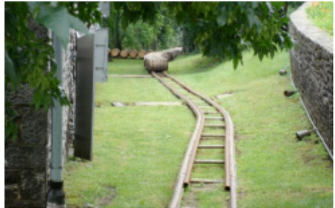
**Photograph 1: Bourbon Barrel Railroad**—The shape of the barrels allows them to easily roll on parallel rails.
