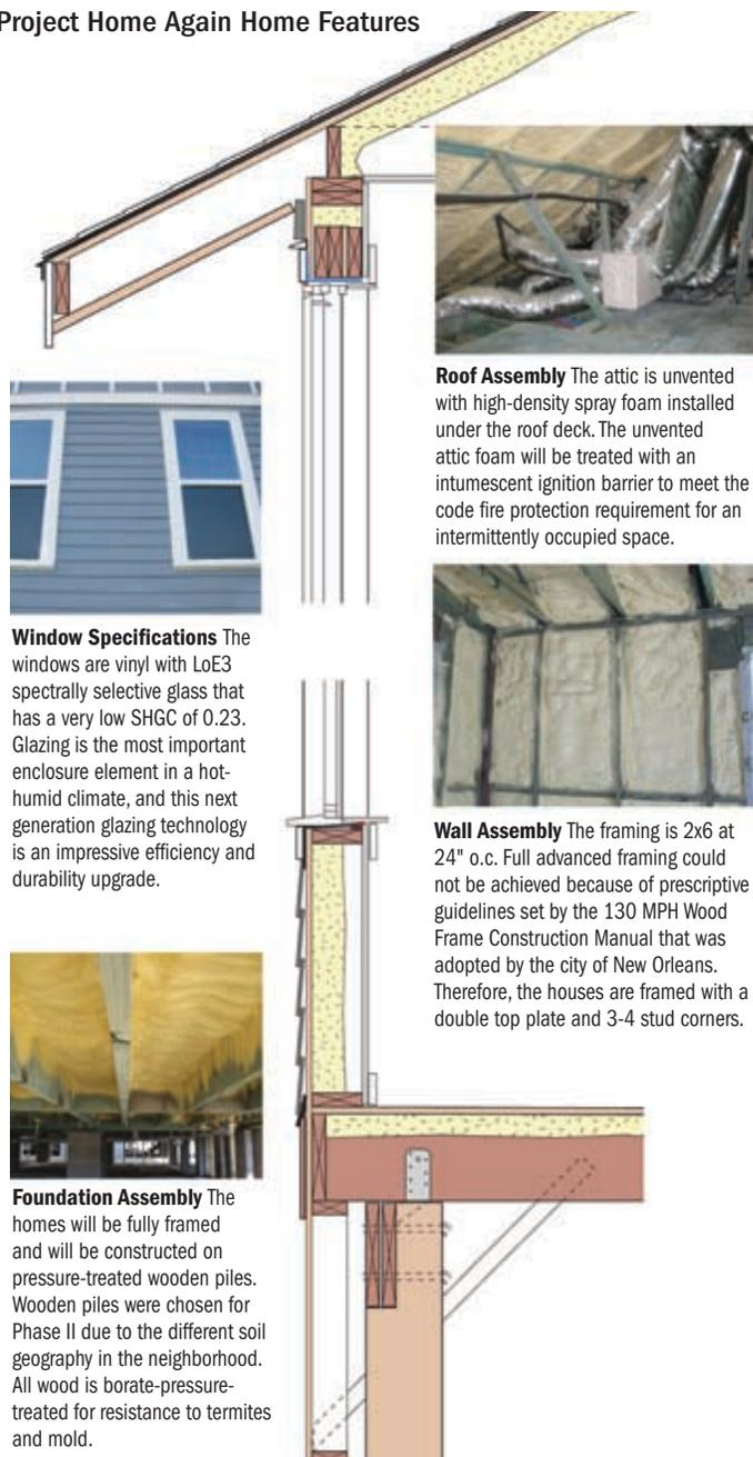
**Roof Assembly** The attic is unvented with high-density spray foam installed under the roof deck. The unvented attic foam will be treated with an intumescent ignition barrier to meet the code fire protection requirement for an intermittently occupied space.
