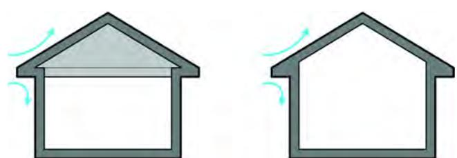
**Figure 2** *Unvented cathedralized attic (left) and unvented cathedral ceiling (right) assemblies.*
