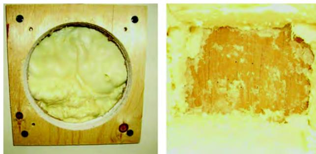
**Figure 12** Jig and core through drywall (left) and foam cut to interior face of plywood (right).
