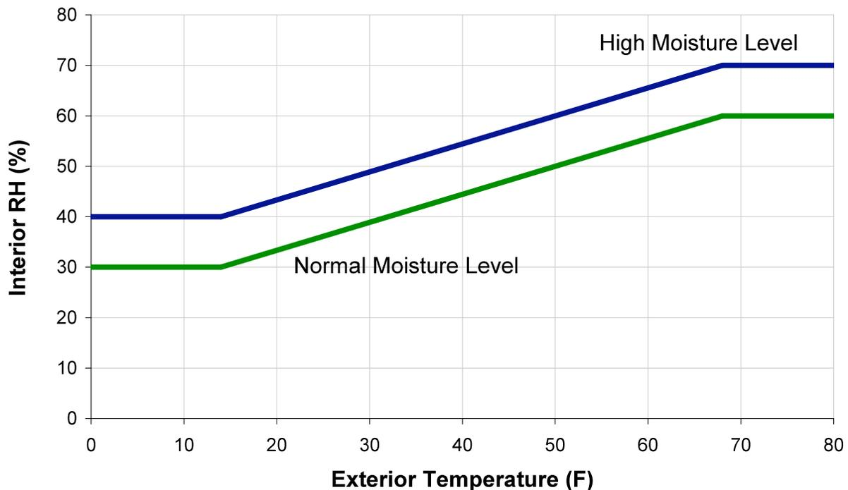
**Figure 4: EuroNorm Standard 15026 Model for Interior RH Levels**
