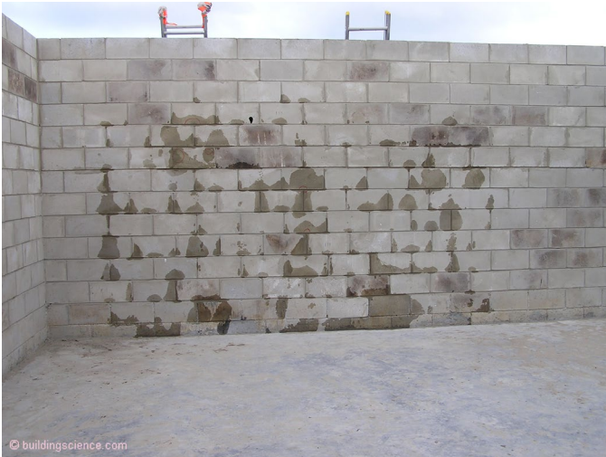
Photograph 5: Pushing Things - Being who I am – I wanted to push things to serious failure. I kept adding water. Long garden hose. Took a little over an hour. It’s why they call me a “hoser”. Neat pattern.
