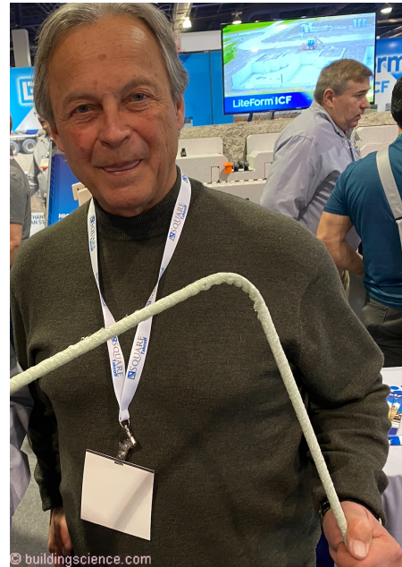
Photograph 4 – Fiberglass Re-Bars - Non-conductive reinforcing bars - awesome. Notice the big smile on the building science guy....
