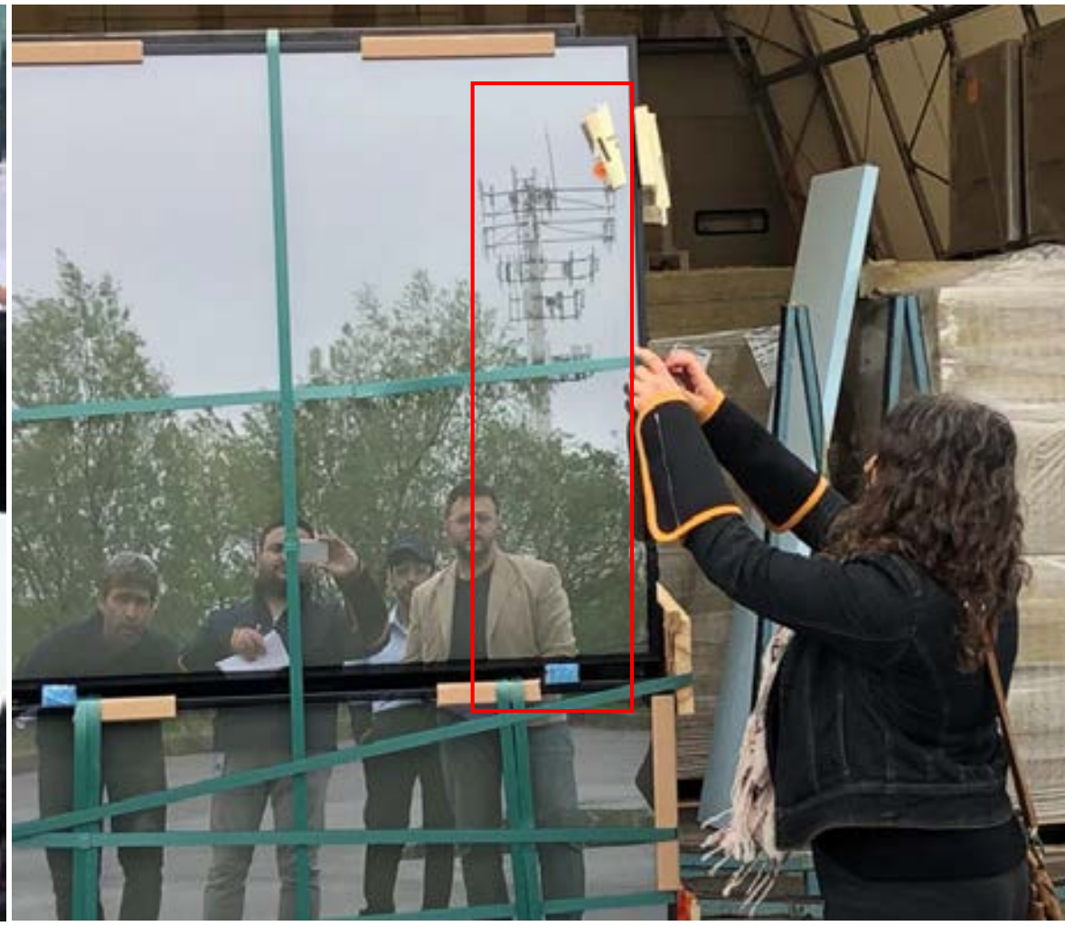
Vertical Roller Wave Distortion
