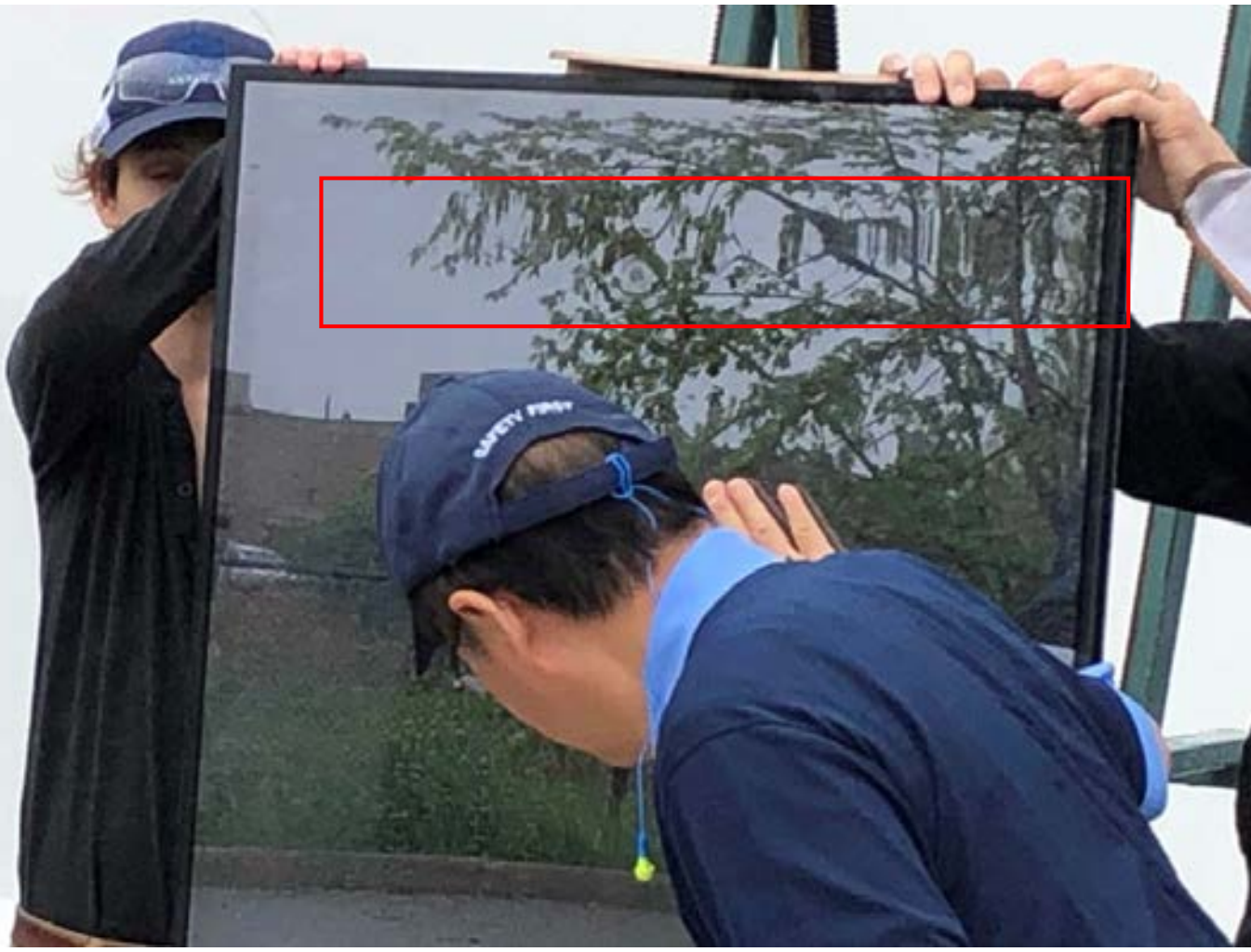
Horizontal Roller Wave Distortion
