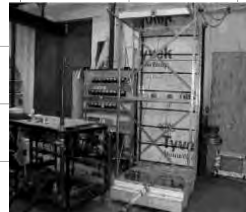
Figure 3. Airflow manifolds connected to test panel on counterbalance system (Burnett et al [2004])
