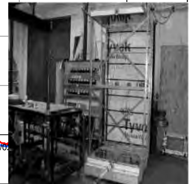
Figure 3. Airflow manifolds connected to test panel on counterbalance system (Burnett et al [2004])
