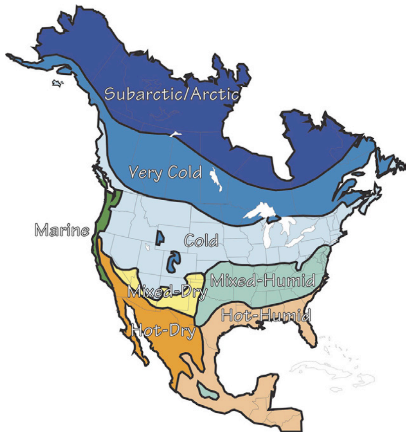
Figure 1: Hygrothermal Regions —From “ BSD-106: Understanding Vapor Barriers ”. You should worry about freeze-thaw in “Cold Climates” (or colder) that have “Moderate” (or higher) amounts of precipitation. Cold Climates are defined more precisely as IECC Climate Zone 5 or higher if you are a Yank.
