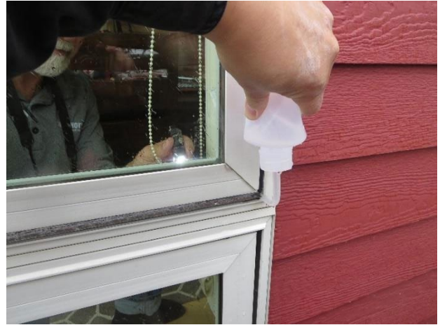
Figure 49: Water squirt bottle injecting water
