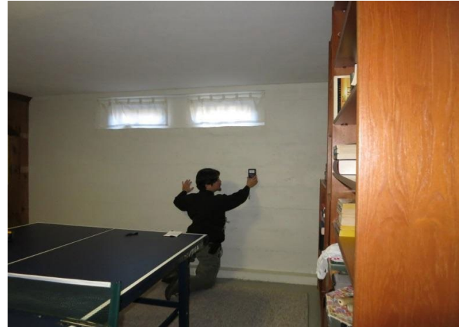
Figure 24: Tramex moisture meter measurement of CMU basement wall
