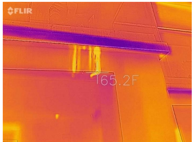
Figure 56: Visual and infrared image of correctly-draining glass railing detail (drainage gap)
